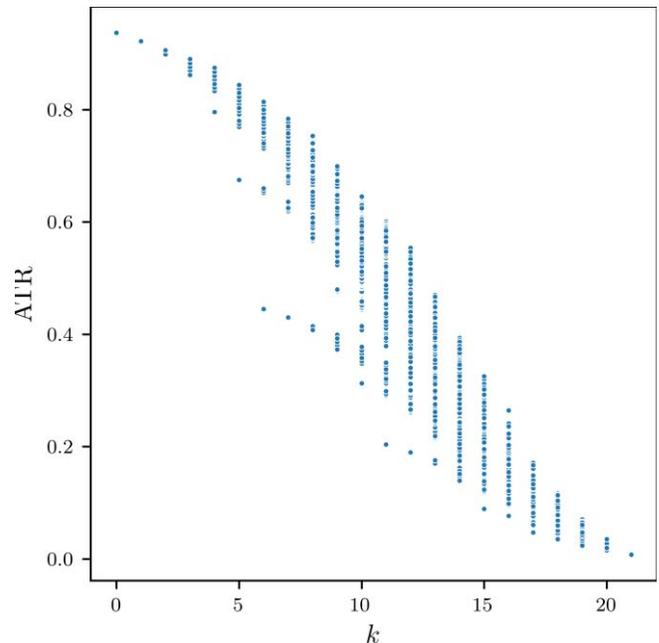
Figure 3. The  $N - k$  full-spectra all-terminal reliability for the 8-node complete graph with 50% edge failure probability.
